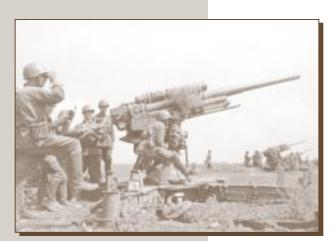
A battery of Russian ZP39 85mm anti-aircraft guns. Although originally designed solely for the anti-aircraft roll, the ZP39—like its German counterpart, the FlaK 43 8.8cm AA gun—found much favor on the front lines as an antitank gun. Its high velocity 85mm rounds were devastating against even the heaviest of German armor.
